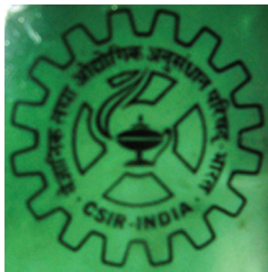
Figure 2. Clear transparent green film of PPC blend. [Color figure can be viewed in the online issue, which is available at wileyonlinelibrary.com.]
